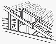
In structures that have a space between the ceiling and the roof such as an attic or crawl space, a light tunnel must be built. Nailers of 2" x 4" must be used to frame the opening between the roof header and the ceiling header. These will be used for attaching the finishing material, i.e., drywall, wall board, plywood, etc. The light tunnel should be wrapped with insulation for optimum performance. Select the desired shaft, and frame accordingly.
