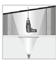
STEP 5 - On the roof, locate the centering hole and outline the diameter of the hole that the pipe will pass through by turning the flashing (E) upside down and marking the inside of the flashing unit.
